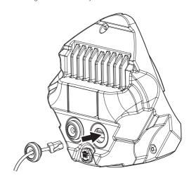
2-4. Connect the network cable jack to the PoE port of the camera body.
