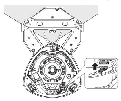
7. Using the fastening screws on the camera body, fix the camera body to the mount bracket.
