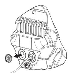
5. Insert the cable bushing of the audio/alarm cables into the camera body.
