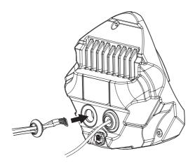
6. Connect the audio/alarm cable connector to the audio/alarm cable port of the camera body.
