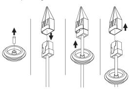
2-3. Mount the cable bushing to the camera body.
