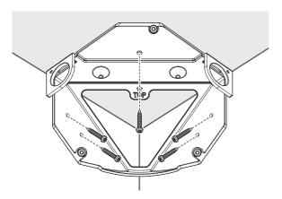
1-3. Pull out network cable through the hole in the mount bracket.
