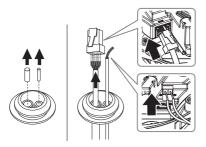
**3-4.** Mount the cable bushing to the camera body.
