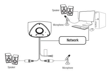
Connect the MIC port of the camera with the microphone or LINE OUT port of the amplifier that the microphone is connected to.
