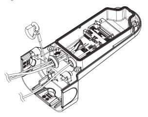
4-2. Connect the connector of the audio/alarm cables to the Audio/Alarm port.
