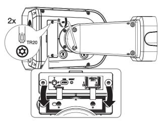
2. Insert a Micro SD card in the direction of the arrow.
