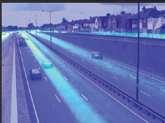
You can activate a motion Heatmap to highlight in your image the most move-mented areas. The system will save a snapshots of the heatmap every X seconds configured like the example on the left:
