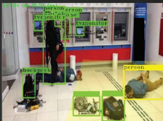
With object Orientation filter you can trigger alarms only if your target object is in a horizontal position like the yellow object in the image on the left:
