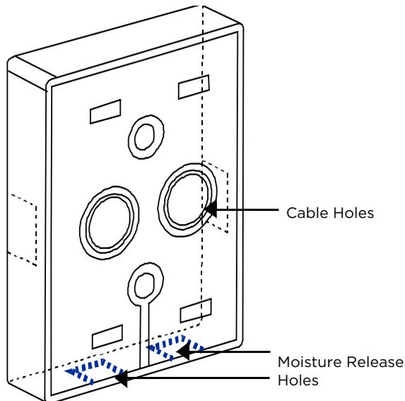
2. Position and secure the antenna backplate to the mounting surface so that the two moisture release holes are on the bottom.
