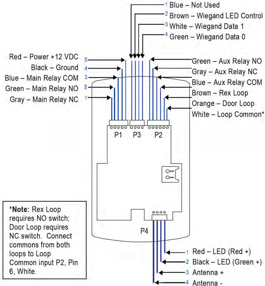
The main relay for the door-locking device is wired to connector P1 on the EntryProx main circuit board.
