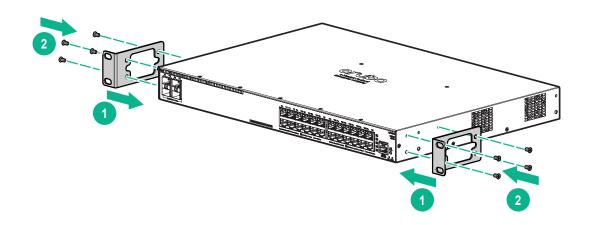
**2.** Use the four number 12–24 screws to secure the brackets to the rack.
