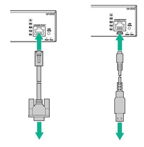
**NOTE:** If both cables are connected, input is accepted only from the Micro USB connector. For more information, see the information on connecting a management console in the **Aruba 2930F Switches Installation and Getting Started Guide**.
