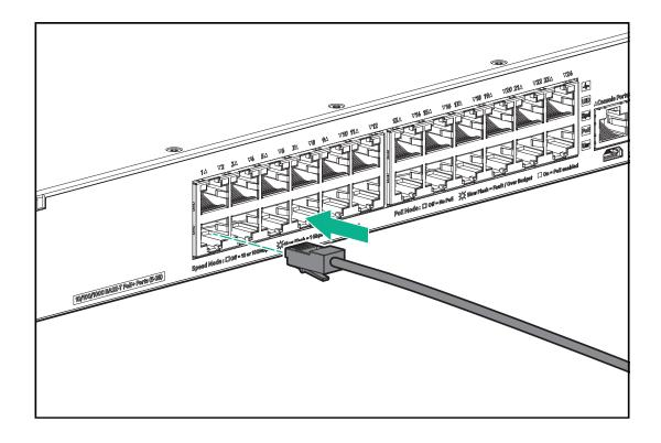
**NOTE:** In the factory default configuration, the switch automatically obtains its IP network settings from a DHCP or BootP server after connecting to the network. If you do not use direct console access to initially determine the switch IP address, you can determine the assigned IP address by inspecting your DHCP/BootP server or by querying LLDP information from another, directly connected neighbor switch. CLI LLDP commands for an ArubaOS neighbor switch are listed below.
